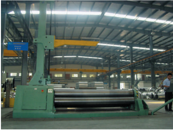
进口全自动微机控制4辊卷板机(瑞典) The Fully Automatic Micro-processor Control Bending Machine with 4 Rollers (Imported from Sweden)
