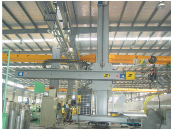
进口全自动环缝焊接工作站(瑞典) The Fully Automatic Ring-seam Welding Station (Imported from Sweden)
