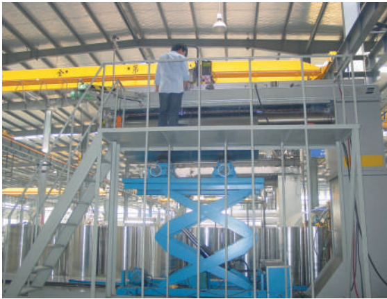
进口全自动纵缝焊接工作站(瑞典) The Fully Automatic Vertical-seam Welding Station (Imported from Sweden)
